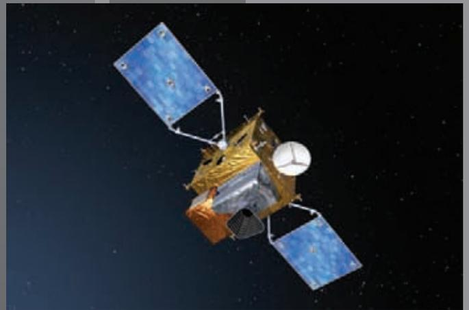
↑ The Sentinel-4 mission consists of two instruments carried on the Meteosat Third Generation Sounder satellite, to be launched in 2019
