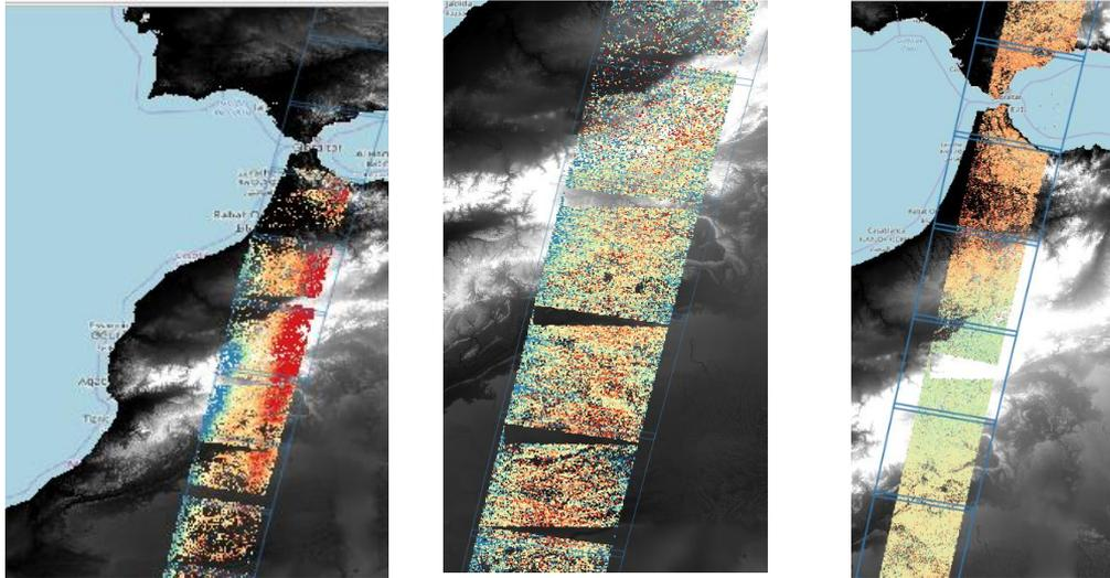
**Figure 5-4: Visual analysis for a selection of the sensor twins as the GLS/LM5 across track (left), GLS/LT5 across track (middle) and LS8/S2 across track (right); scale -2.5 pixels red to +2.5 blue pixels @30m.**
