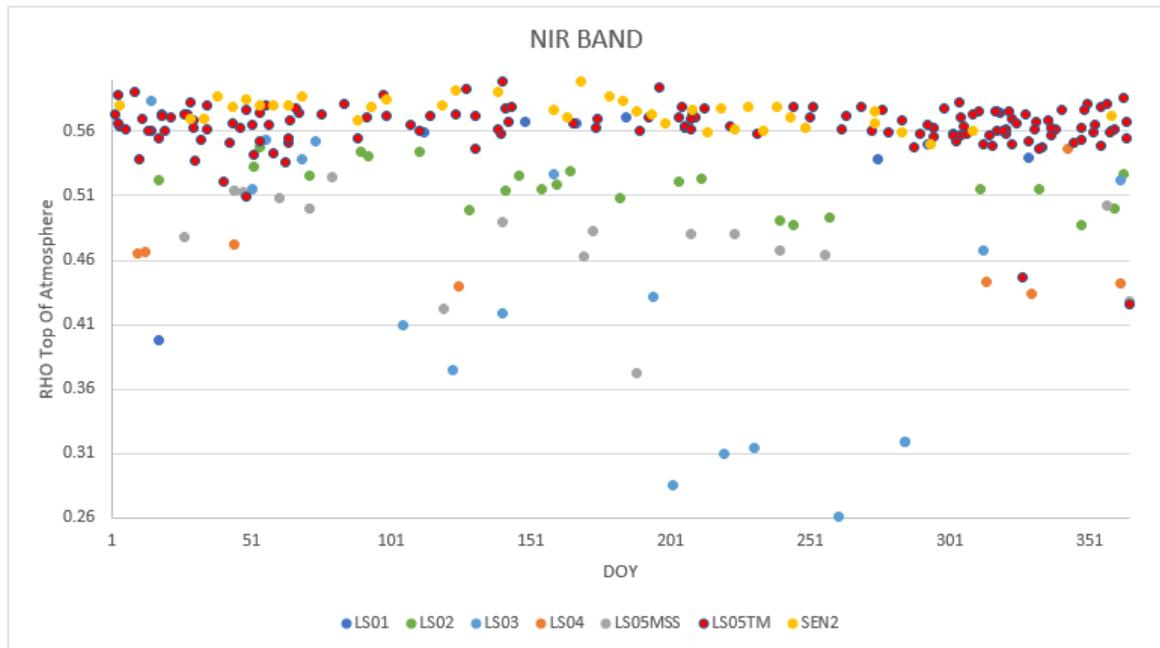
Figure 6-4: Libya1 Landsat 1-5 time-series consistency comparison with Sentinel-2 reference data, NIR Band.
