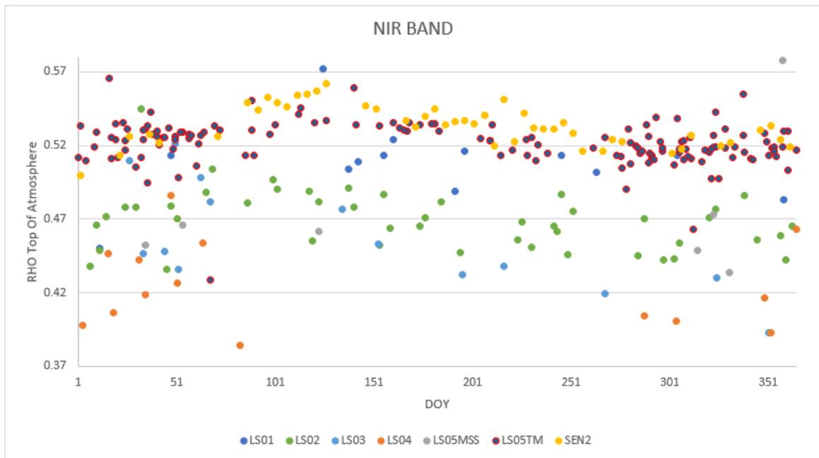
Figure 6-8: Libya4 Landsat 1-7 time-series consistency comparison with Sentinel-2 reference data, NIR Band.
