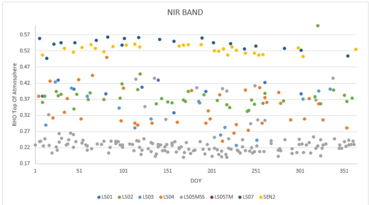
Figure 5-11: Algeria5 Landsat 1-5 time-series consistency comparison with Sentinel-2 reference data, NIR Band.
