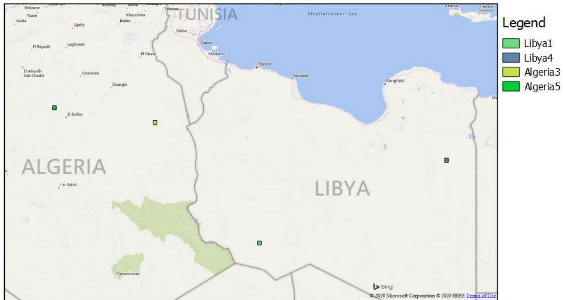
Figure 5-7: Spatial distribution of PICS used for the radiometric assessment, each Region of Interest half a degree in height and width.
