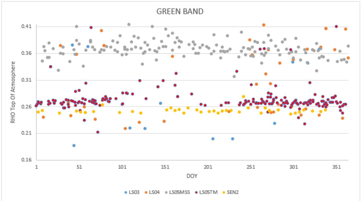
Figure 6-10: Algeria3 Landsat 3-5 time-series consistency comparison with Sentinel-2 reference data, Green Band.
