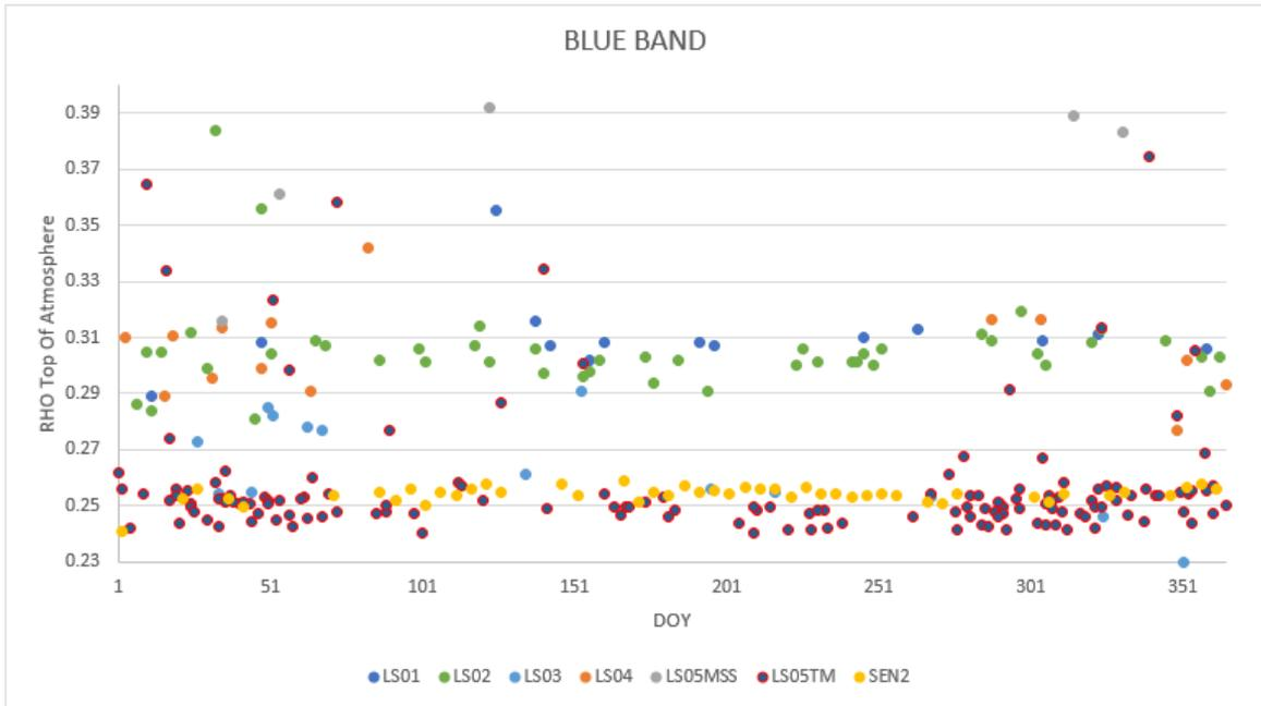
Figure 6-5: Libya4 Landsat 1-7 time-series consistency comparison with Sentinel-2 reference data, Blue Band.
