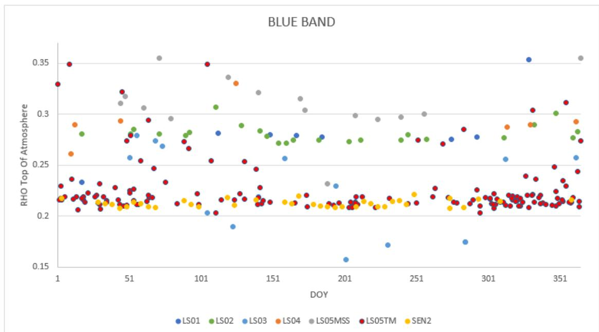
Figure 6-1: Libya1 Landsat 1-5 time-series consistency comparison with Sentinel-2 reference data, Blue Band.
