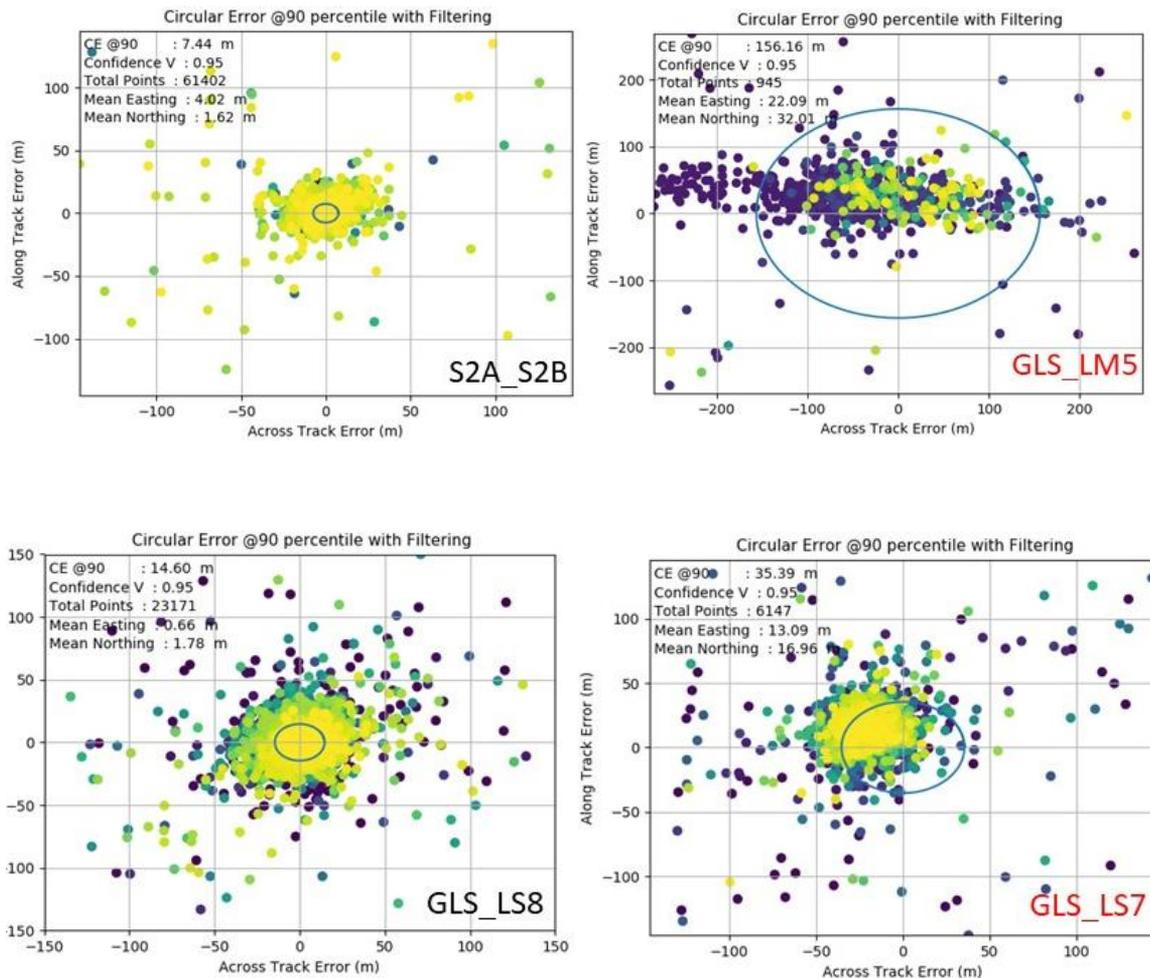
Figure 5-3: Circular Error plots for a selection of the sensor twins.
