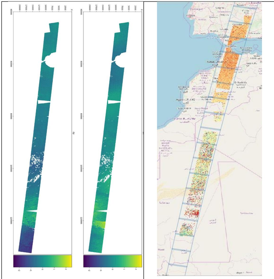
Figure 5-5: S2/LS08, across (left) and along track (middle) displacements (scale: +/- 2.5 pixels @30m) with the location shown (right) as S2A/B across track differences (scale -2.5 pixels red to +2.5 blue pixels @30m).
