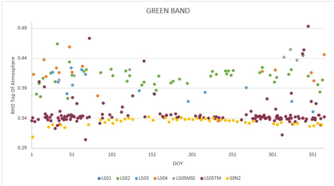
Figure 6-6: Libya4 Landsat 1-7 time-series consistency comparison with Sentinel-2 reference data, Green Band.
