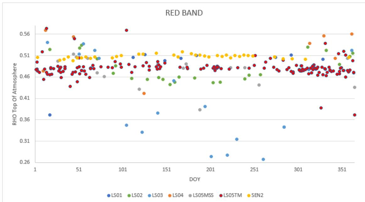
Figure 6-3: Libya1 Landsat 1-5 time-series consistency comparison with Sentinel-2 reference data, Red Band.
