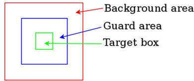
Figure 2: Example of basic geometry for CFAR sliding window
