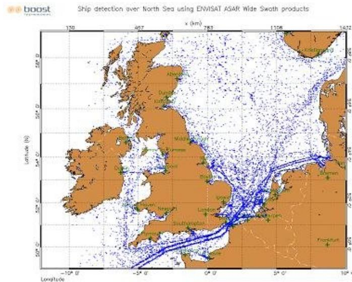
Figure 7: Ship detection over Europe using ENVISAT ASAR Wide Swath products (Channel)
