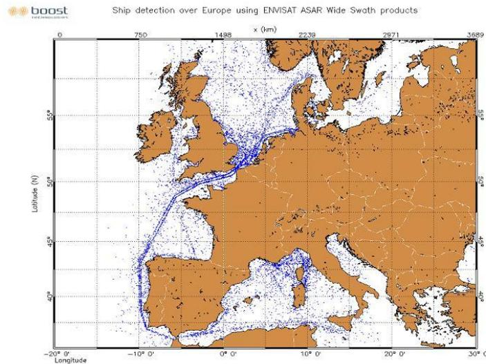
Figure 4: Ship detection over Europe using ENVISAT ASAR Wide Swath products (Overview)
