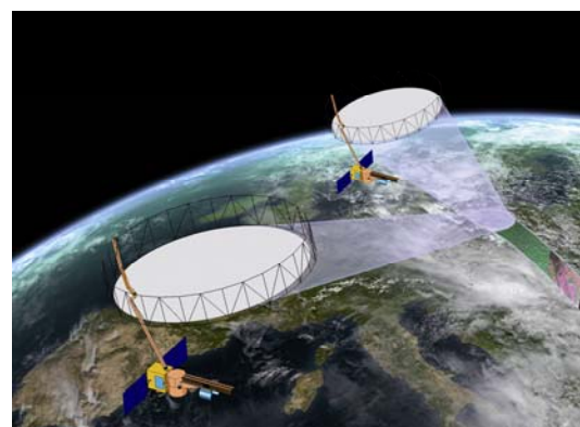
Figure 7: Artistic view of a Tandem-L formation with two satellites (preliminary design achieved during a joint DLR and NASA/JPL pre-phase A study).
