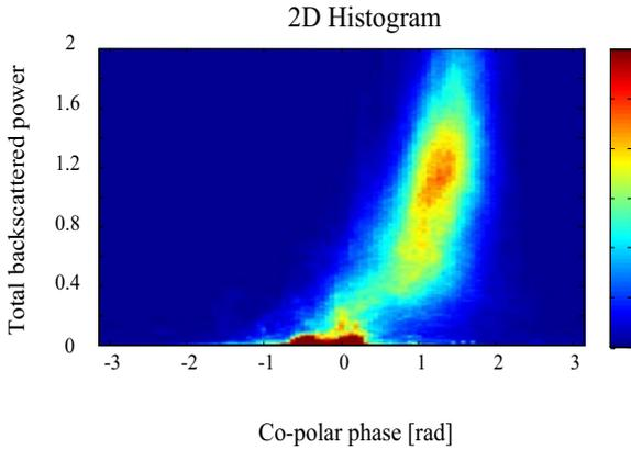
Fig. 2. Joint distribution of the total backscattered power and the co-polar phase for the co-polar channels. The total backscattered power has been obtained as the sum between the HH and VV backscattered powers. The color scale is proportional to the number of counts within each bin.
