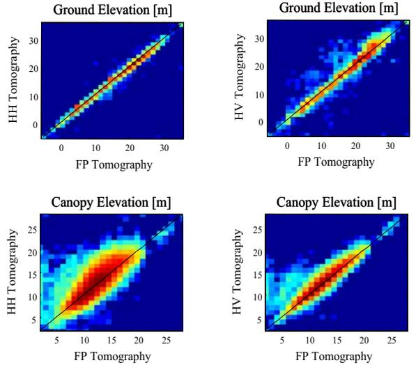
Fig. 8. Joint distribution of the elevation estimates yielded by processing the single channels separately (vertical axis) and by the best tomography (horizontal axis). The black line denote the ideal linear trend. The color scale is proportional to the natural logarithm of the number of counts within each bin.
