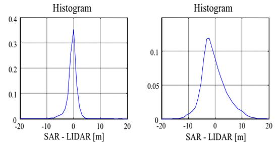
Fig. 5. Histograms of the differences of the elevation estimates relative to the ground and the canopy yielded by T-SAR and LIDAR measurements.
