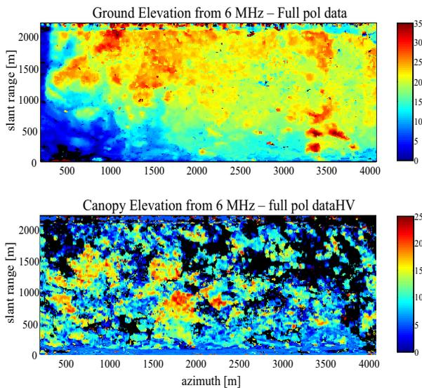
Fig. 9. Top row: estimated ground elevation. Black areas correspond to an unstructured scattering mechanism. Bottom row: estimated canopy elevation. Black areas correspond to absence of canopy.
