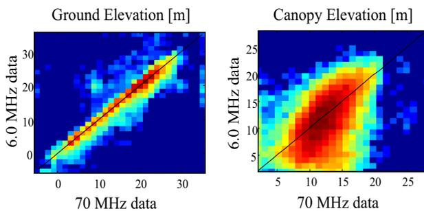
Fig. 10. Joint distribution of the elevation estimates yielded by processing the 6 MHz data (vertical axis) and by the best tomography (horizontal axis). The black line denote the ideal linear trend. The color scale is proportional to the natural logarithm of the number of counts within each bin.
