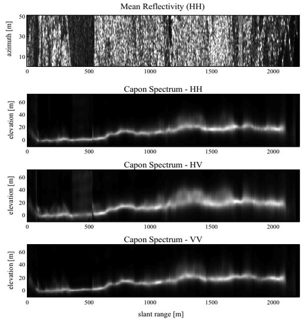
Fig. 3. Top panel: mean reflectivity of the data (HH channel) within a stripe as wide as 50 m in the azimuth direction. The underlying panels show the Capon Spectra for the three polarimetric channels. At every range bin the signal has been scaled in such a way as to have unitary energy.
