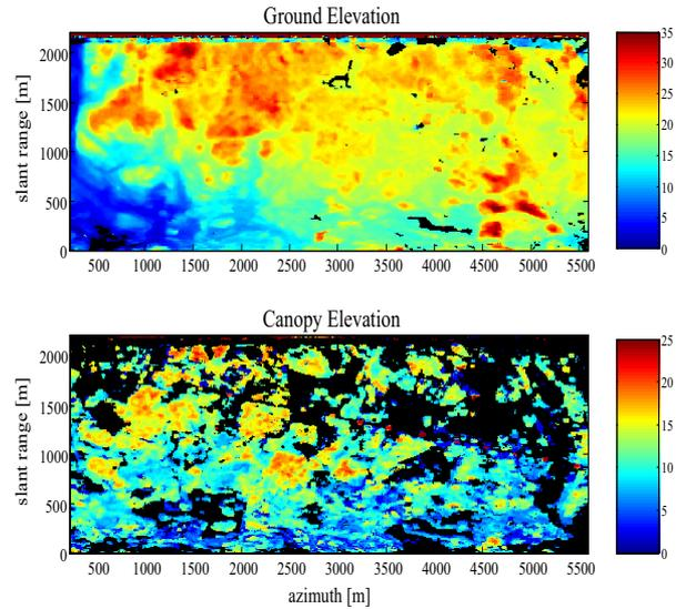
Fig. 4. Top row: estimated ground elevation. Black areas correspond to an unstructured scattering mechanism. Bottom row: estimated canopy elevation. Black areas correspond to absence of canopy.
