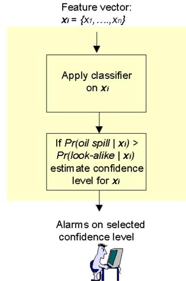
Figure 2. The two-step classification approach.
