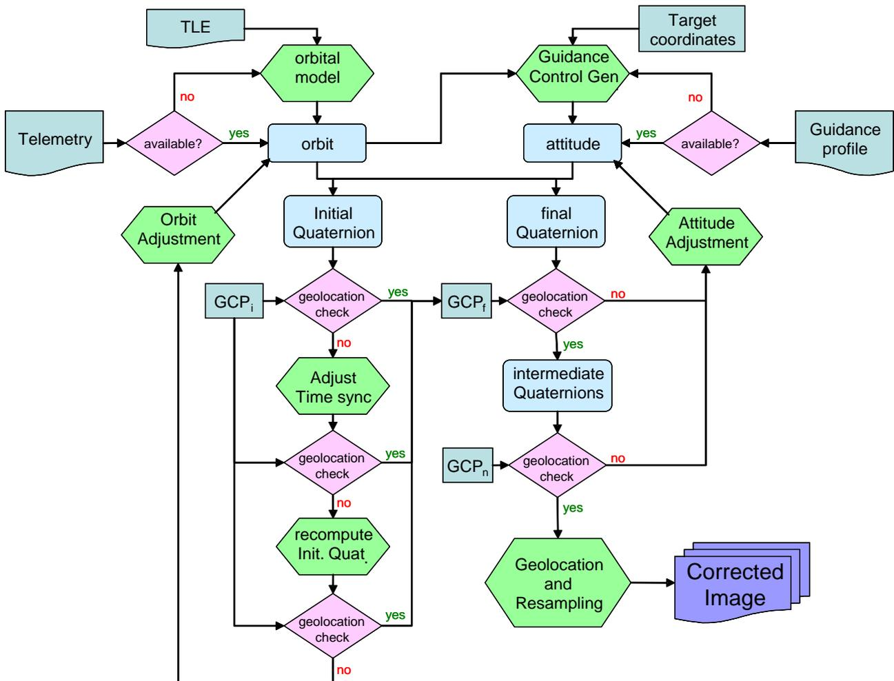
Fig. 7. Flow chart of the parametric algorithm for geometric correction.
