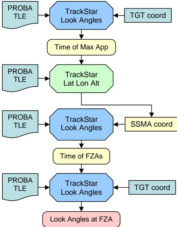
Fig. 2 Flow chart for determination of view angles by orbital propagation.
