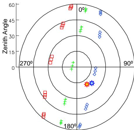
Fig. 6. Polar representation of the calculated observation angles at start, mid and end of each image acquisition.
