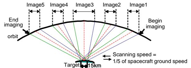
Fig. 5. Scheme of the actual acquisition procedure of CHRIS/PROBA with slowdown factor.
