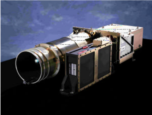
Fig. 5. The Compact High Resolution Imaging Spectrometer (CHRIS)
