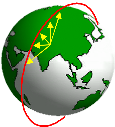
Fig 6. The multi-view angle observation scheme of CHRIS on PROBA
