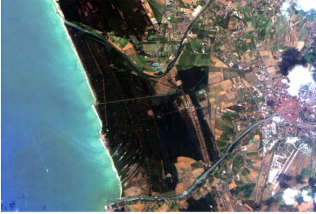
Fig. 3. Reflectance image displayed in “true color”, like in Fig.1, as result of data acquired July 25, 2003 at MZA = -2° and FZA = +36°.
