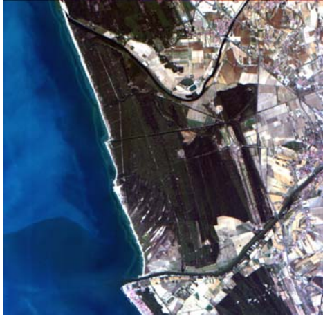
Fig. 2. Same image of Fig.1 after correcting the “stripe-noise”. The vertical lines are strongly reduced.
