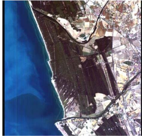
Fig. 1. at-sensor radiance image acquired by CHRIS over San Rossore on September 18, 2003 with MZA =  $-8^\circ$  and FZA =  $0^\circ$ . The image is displayed in "true colors": Red channel (6<sup>th</sup> band, 631 nm), Green channel (3<sup>rd</sup> band, 530 nm) and Blue channel (1<sup>st</sup> band, 442 nm).
