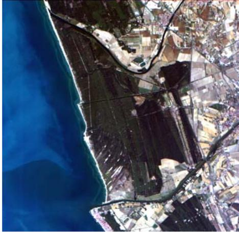
Fig. 2. Same image of Fig.1 after correcting the “stripe-noise”. The vertical lines are strongly reduced.
