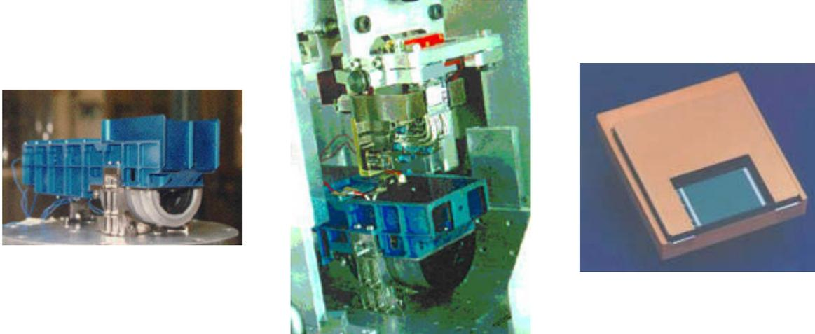
Figure 3.5 - MERIS instrument: camera (left) – spectro-imager camera (centre) – CCD (right).
