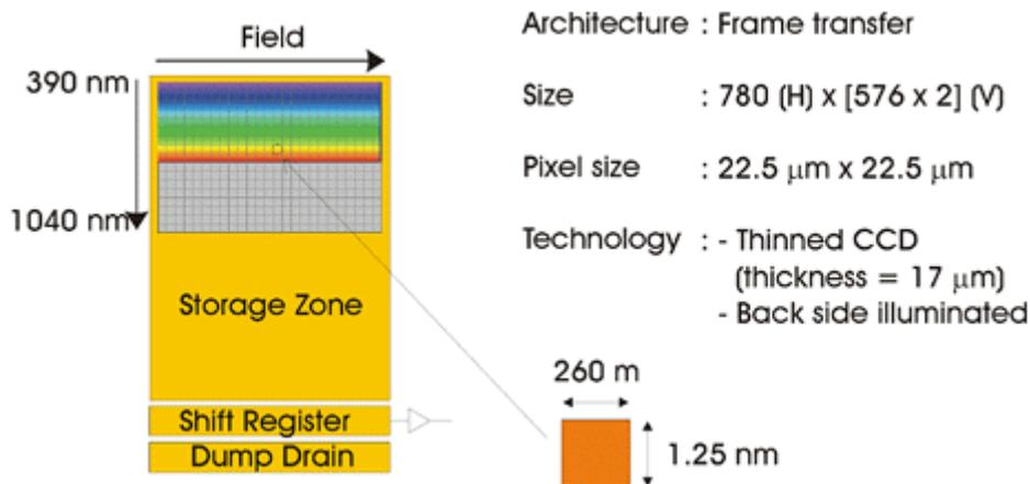
Figure 3.4 - Basic layout of the CCD.
