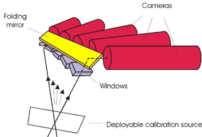
Figure 3.3 - Arrangement of optical modules, folding mirror and Earth viewing windows.
