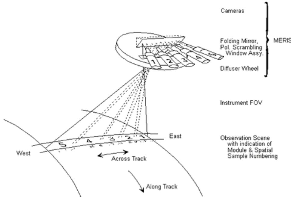
Figure 1.6 - MERIS FOV, camera tracks, pixel enumeration and swath dimension
