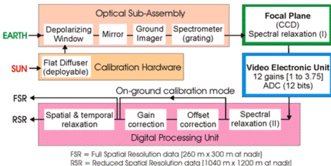
Figure 3.2 - Instrument Concept.
