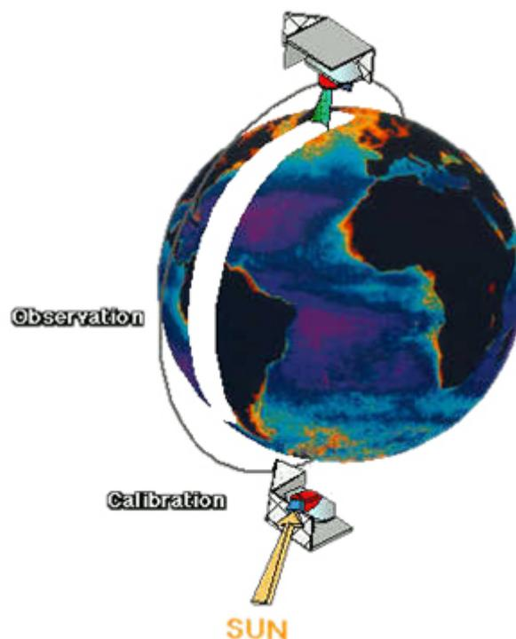
Figure 3.1 - Observation / calibration cycle.
