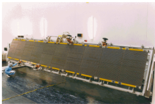
Figure 3.5 ASAR FM antenna after deployment test (Image by courtesy of ASTRIUM Ltd)
