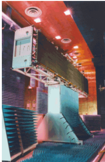
Figure 3.4 ASAR FM antenna during radiation testing (Image by courtesy of ASTRIUM Ltd)
