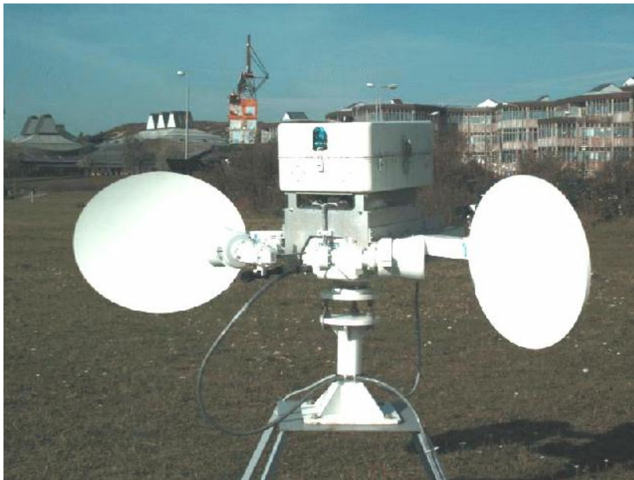
Figure 3.29 Prototype ASAR Calibration Transponder Deployed at ESTEC
