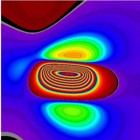
Figure 2. Surface fringe pattern by a 95° strike, 45° dip fault plane.
