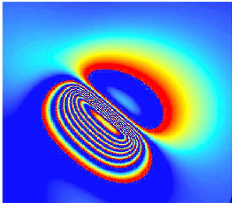
Figure 6. Surface displacement modelled by using the solution from the neural network
