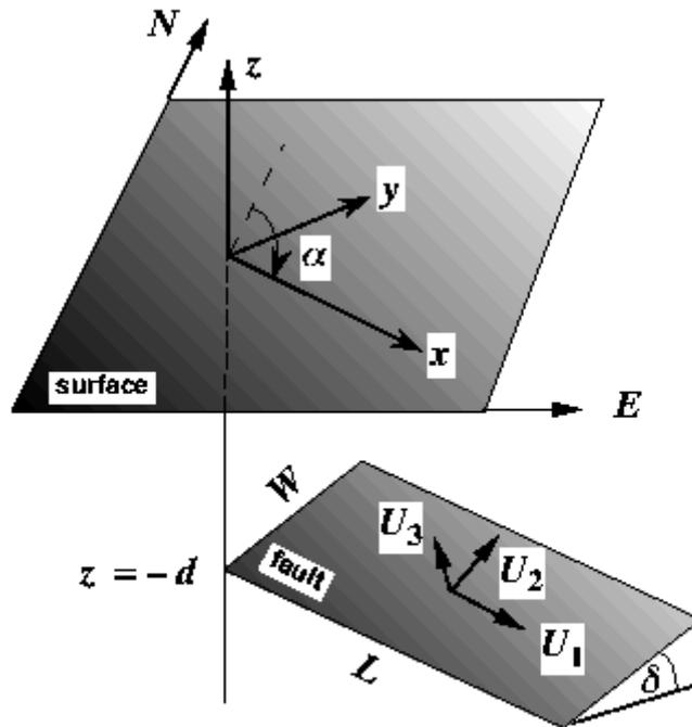
Figure 1. Fault geometry and symbols. The strike ( $\alpha$ ) and dip ( $\delta$ ) angles are shown. The slip vector  $U = [U_1, U_2, U_3]$  represents the movement of the hanging wall with respect to the foot wall oriented such that positive  $U_1$  is left-lateral strike slip, positive  $U_2$  is thrusting dip slip, and  $U_3$  is tensile slip.
