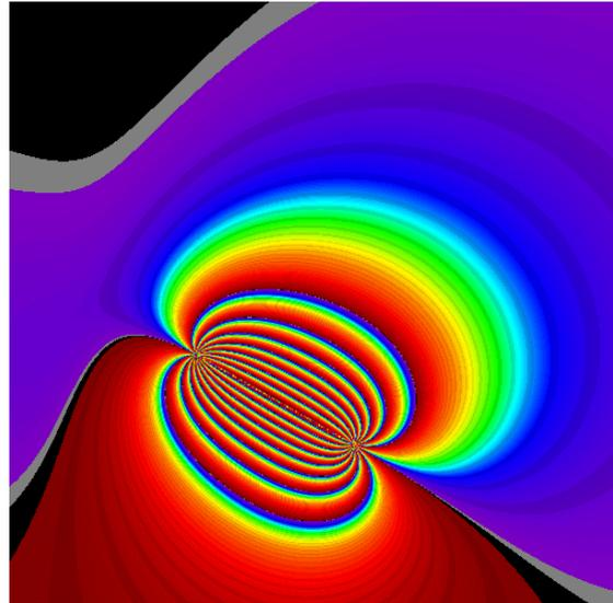
Figure 3. Surface fringe pattern by a 120° strike, 75° Dip fault plane
