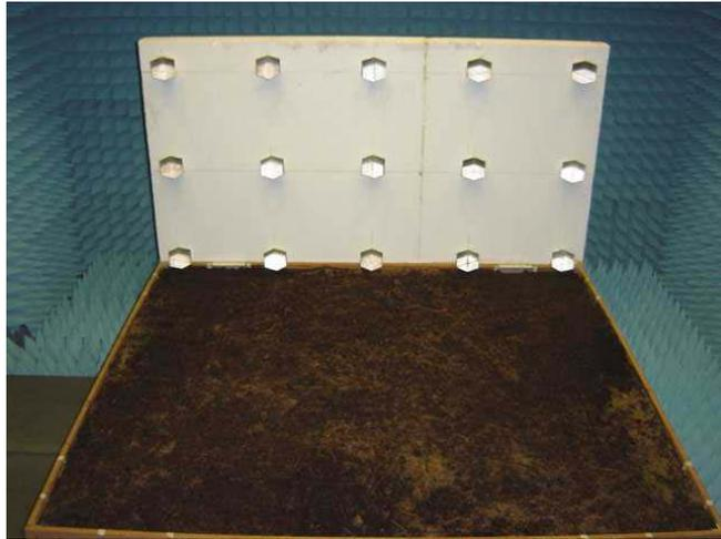
Fig. 3. The position of the trihedral reflectors in the GB-SAR facility
